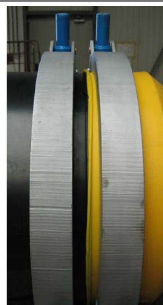
Figure 20: Butt fusion welding
