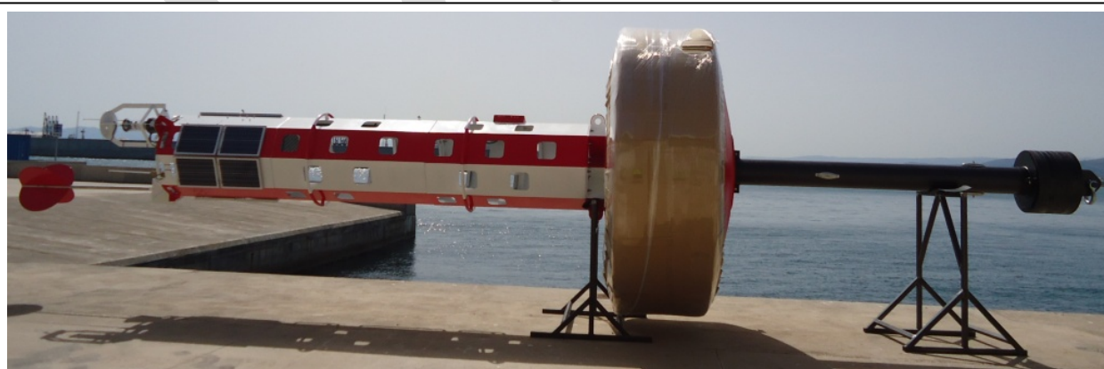
Figure 59: Assembly of an elastomer buoy
