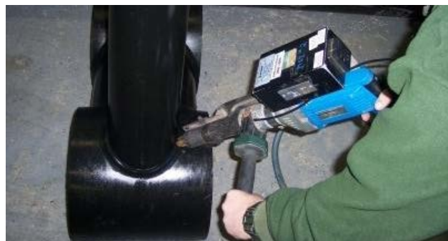
Figure 41: HDPE extrusion welding
