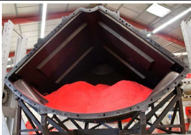
Figure 11: Mould filled with plastic powder
