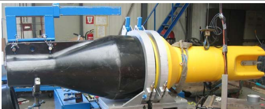
Figure 19: Butt fusion welding
