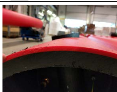
Figure 36: Co-extrusion
